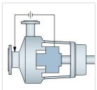
Plan 13 Recirculation from the seal chamber through a flow control orifice and back to the pump suction or pump suction
