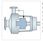
Plan 11 (12) Recirculation from the pump discharge through a flow control orifice (in Plan 12 through a strainer and a flow control orifice) into the seal chamber.
