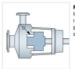
Plan 01 Integral (internal) recirculation from the pump discharge to the seal chamber
