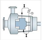
Plan 23 Recirculation from a circulation device in the seal chamber through a cooler and back into the seal chamber.
