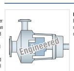
Plan 99 Engineered piping plan not defined by other existing plans.
