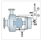
Plan 53A Pressurized barrier fluid reservoir supplying clean fluid for an arrangement 3 pressurized dual seal.
