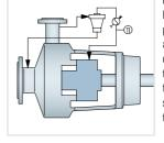
Plan 41 Recirculation from the pump discharge through a cyclone separator delivering the clean fluid to a cooler and then to the seal chamber. The solids are delivered to the pump suction line.
